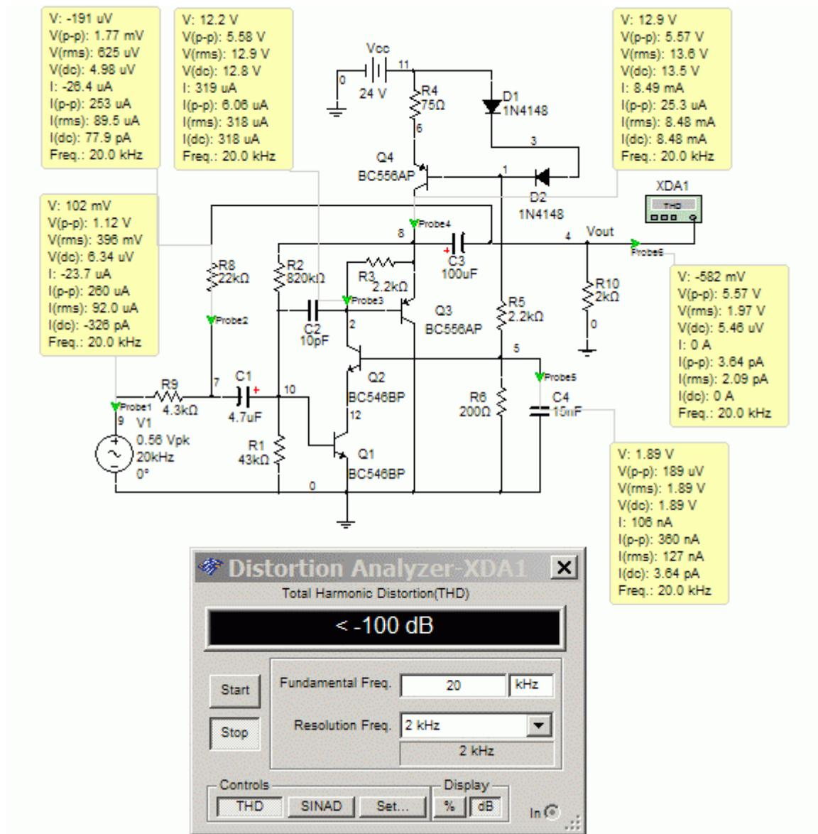
Fig.13-14. Simulation of the inverting amplifier circuit at 20Hz and 20kHz.
