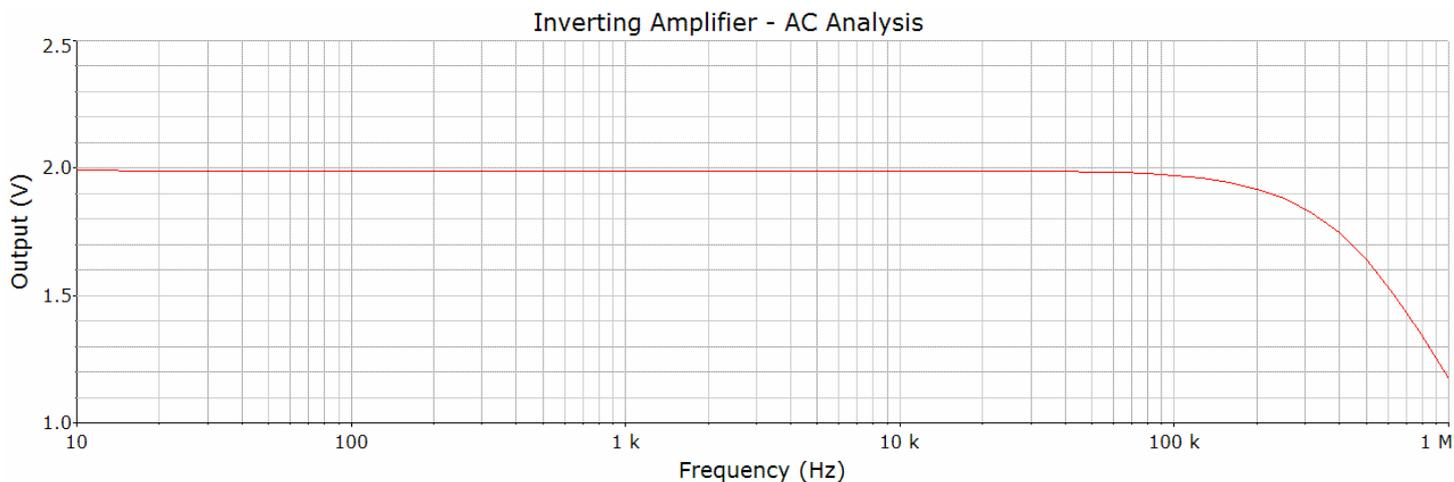
Fig.9. AC analysis of the inverting amplifier with feedback.
