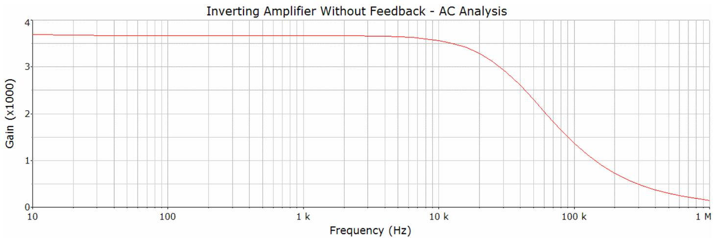
Fig.6. Inverting amplifier open-loop gain.
