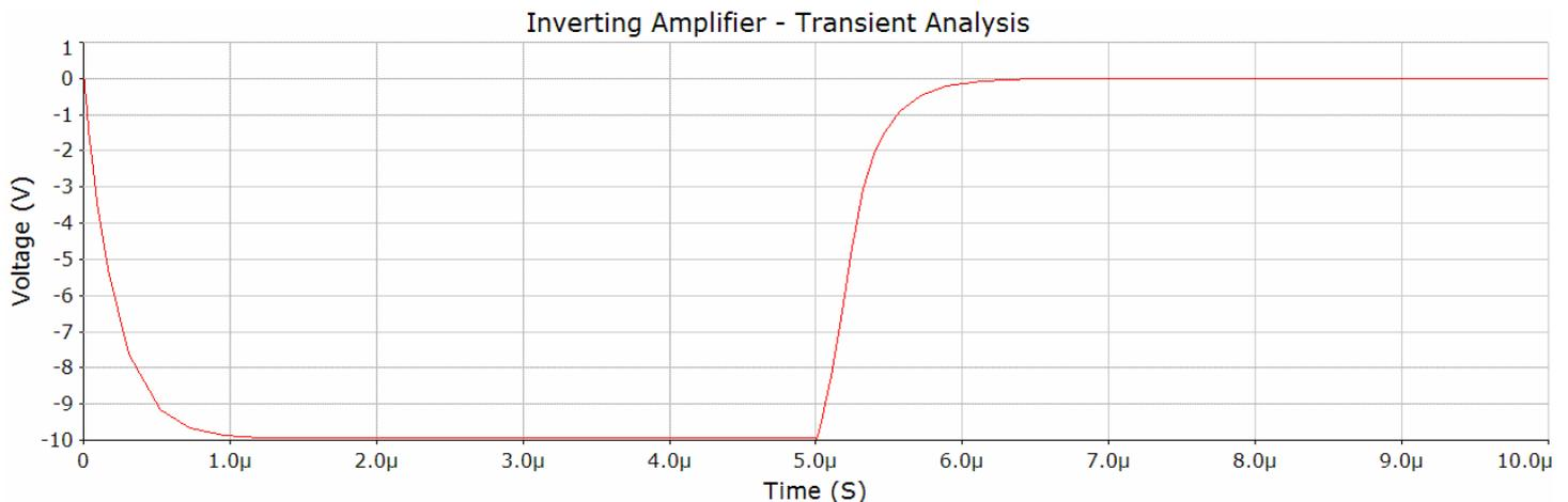
Fig.17. Transient analysis of the inverting amplifier with feedback.
