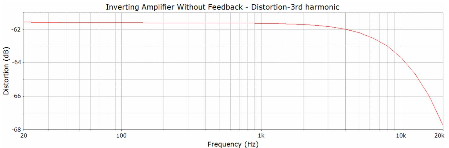
Fig.7-8. Inverting amplifier distortion.
