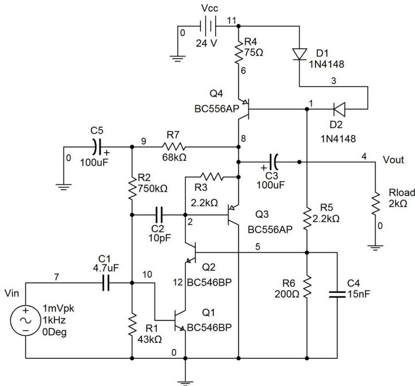
Fig.5. Inverting amplifier without feedback.
