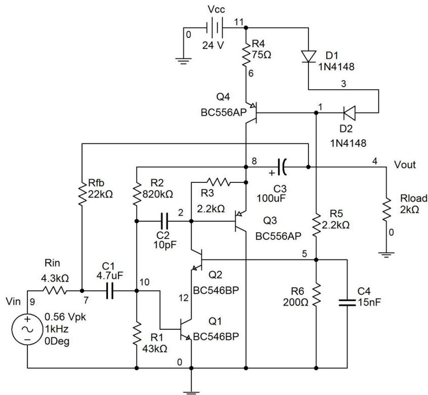
Fig.2. Inverting amplifier with feedback.
