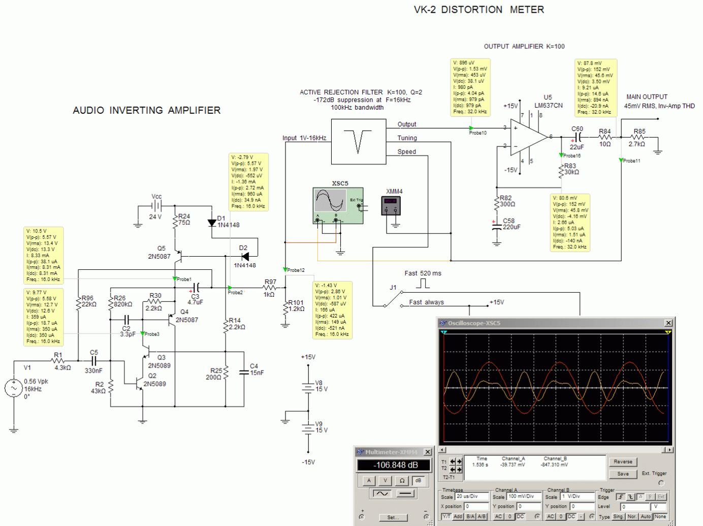
Fig.15. VK-2 distortion measurement of the inverting amplifier at 16kHz.
