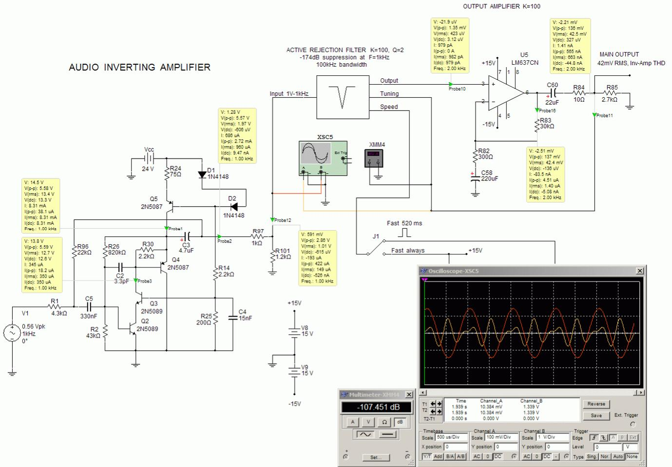
Fig.16. VK-2 distortion measurement of the inverting amplifier at 1kHz.
