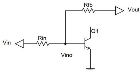
Fig.3. AC equivalent input circuitry of the inverting amplifier.
