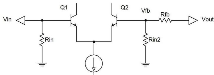
Fig.4. AC equivalent input circuitry of the differential amplifier.
