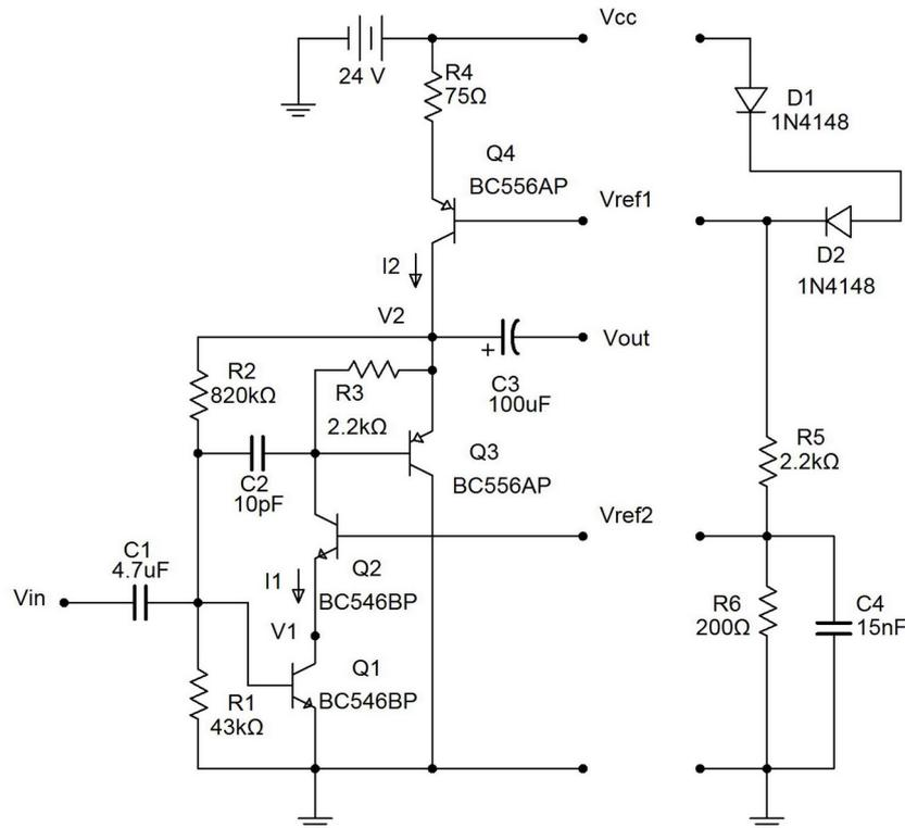
Fig.1. Basic inverting amplifier configuration.
